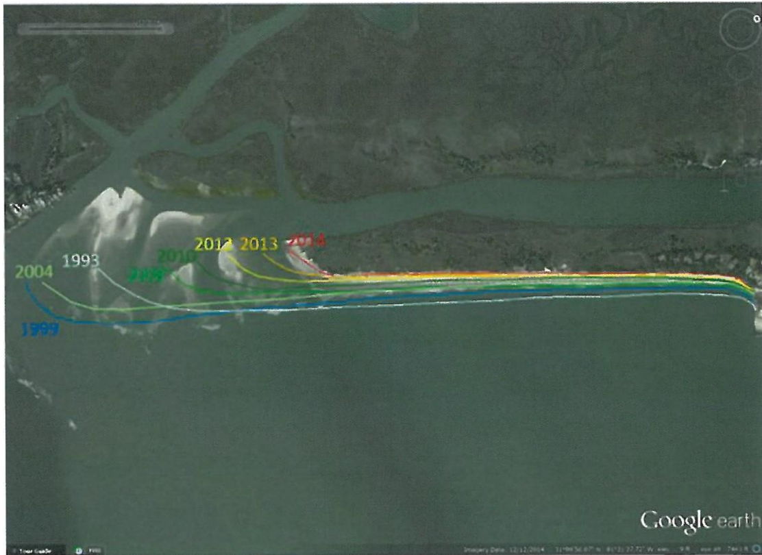
Figure 2: Digitized shorelines from a series of aerial images from Google Earth. After the construction of the south groin in 1990 the spit continues to extend south until approximately 1999. Chester Jackson at GSU has documented the southward extension of the spit since 1869. Since 1999, the south end of the island has been rapidly retreating, reversing a 130-year trend. The entire oceanfront shoreline has also retreated significantly. Inlet dynamics may play some role in the changes at the spit, but there is no question that the large deficit in longshore sediment transport caused by the trapping of sand behind the existing groins has also played a significant role. And the groin must be assumed to be entirely responsible for the rapid erosion of the beach along the oceanfront. Another groin, as proposed in this project, will simply exacerbate the existing, rapid decline on the south end of the island.
